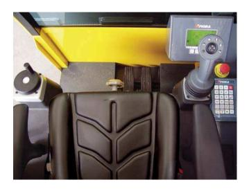
The control centre features a large LCD which displays the actual wheel angles, the selected steering and travel modes of operation.
